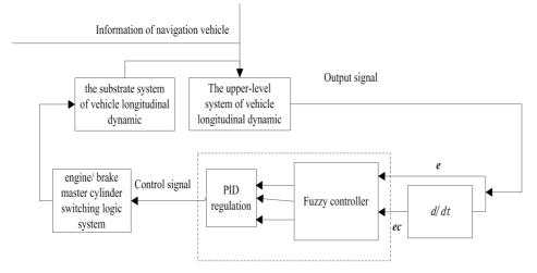
Fig. 1. The longitudinal dynamic fuzzy PID control system of automobile
